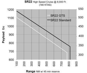
+1 lb (.45kg) Payload or Equipment = - 1.7 NM 75% to 55% PWR = + 40% Range
