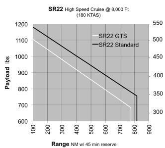
+1 lb (.45kg) Payload or Equipment = - 1.7 NM 75% to 55% PWR = + 40% Range
