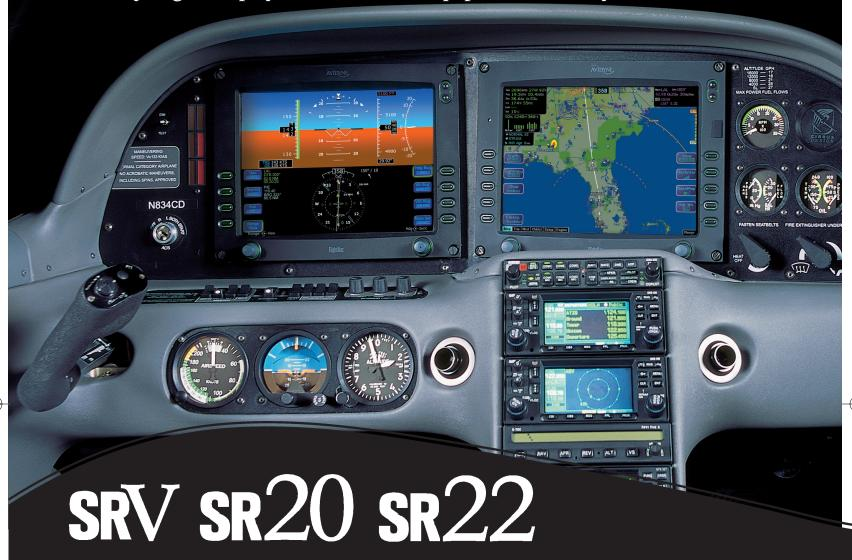
CIRRUS is the first personal aviation manufacturer to deliver the Primary Flight Display [PFD] and Multi-Function Display [MFD] as standard equipment on every model. The Avidyne FlightMax® Entegra PFD and MFD makes flying safer and more intuitive by improving situational awareness.
