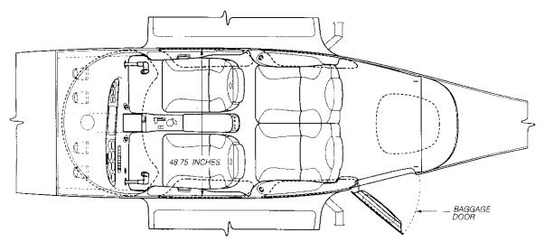
The monocoque fuselage is constructed primarily of composite materials. The design is optimized to reduce skin friction drag and to prevent flow separation. All flight and static loads are transferred to the fuselage skin structure. The main wing spar carry-through is attached to the fuselage in two locations and sits under the two front seats. The rear spar is attached to the fuselage side-walls, just aft of the rear seats.
