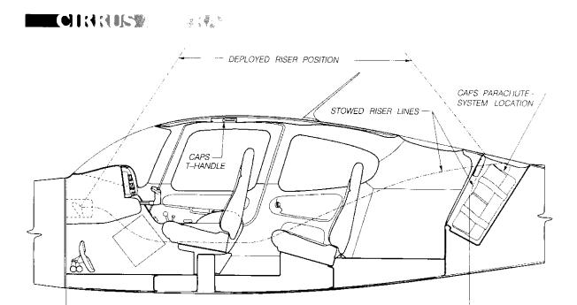
The Cirrus Airframe Parachute System (CAPS) is located in a canister within the fuselage directly behind the cabin's aft baggage bulkhead. It is ready to deploy in order to decelerate and lower the entire aircraft, should controlled flight become impossible. The parachute will deploy only after the pilot or a passenger removes a placarded cover and then pulls a T-shaped activation handle located on the ceiling of the cabin. This two-step process prevents accidental activation.
